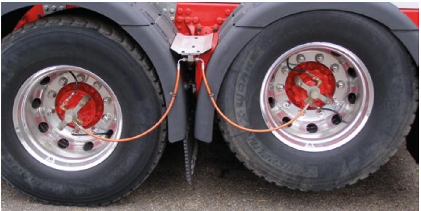
Tyre pressure control systems fitted to timber lorries can help reduce the impact on fragile roads.
