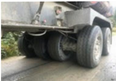
This bespoke low ground pressure timber vehicle spreads the weight of the load across the road.
